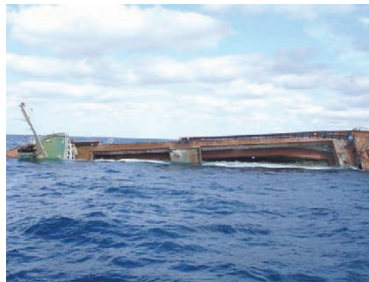
Sinking The Ophelia Brian off Key Biscayne, Miami, Florida. Originally a 210 foot long freighter built in 1965, environmentally cleaned by Bruce Schurger & Company.
